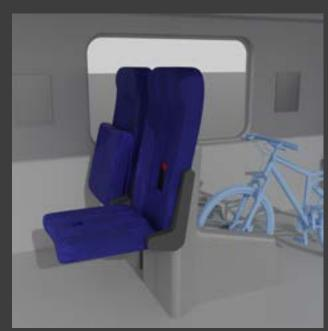
The passenger inserts a bike wheel into a slot at the rear of the seat, the bike weighs down a pressure plate, and the seat is unlocked and able to be folded down to sit on. I initially developed three designs, of which I would end up using two, one allows the passenger to store their bike upright, creating more space, and the other allows the passenger to store their bike with both wheels on the floor, making it more accessible.
